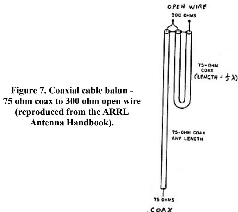
**Figure 7. Coaxial cable balun - 75 ohm coax to 300 ohm open wire (reproduced from the ARRL Antenna Handbook).**
