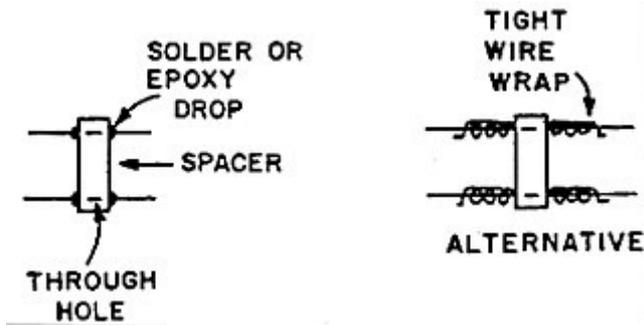
Figure 10. Insulating spacers fitted to open wire line. (reproduced from the ARRL Antenna Handbook).
