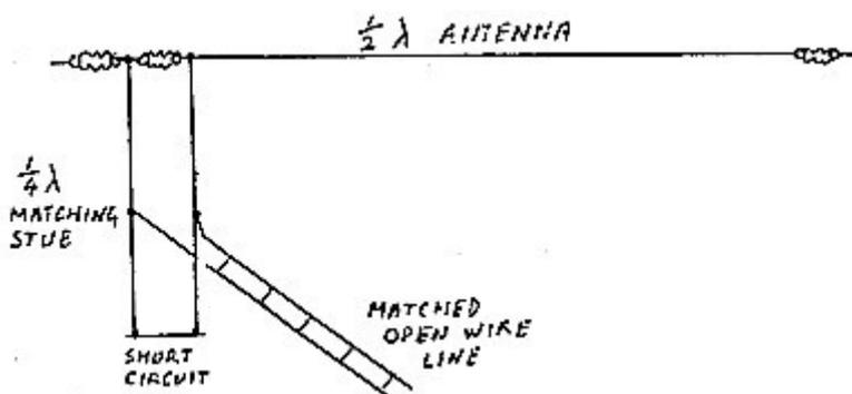
Figure 5. End fed half-wave antenna fed with open wire line and matched using a quarterwave stub.
