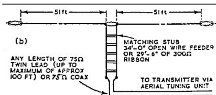
Figure 3. The G5RV antenna with 75 ohm transmission line.
