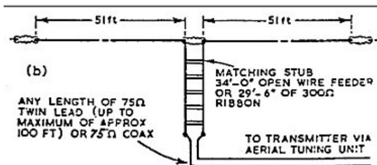
Figure 3. The G5RV antenna with 75 ohm transmission line.
