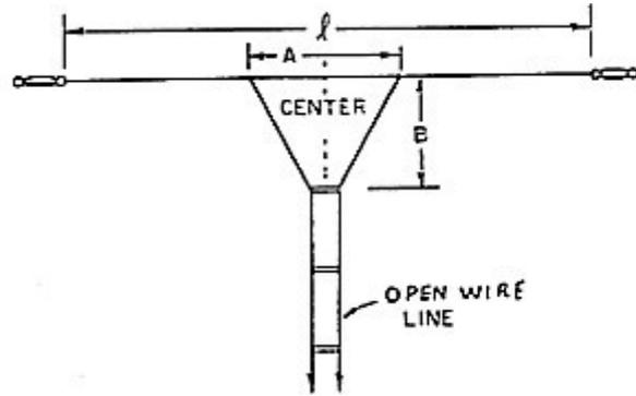
Figure 9. Delta match for balanced line.
