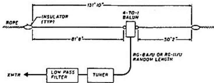
Figure 4. The The Carolina series fed Windom antenna using coaxial transmission line.
