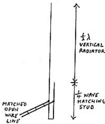
Figure 8 The "J" antenna with matching for open wire or other balanced line.
